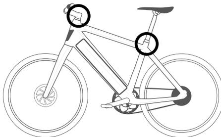
Positions of screw connections for adjusting the sitting position
