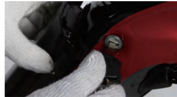
Before loading the battery, please make sure the key lock is in unlocked position. To secure the battery, please turn the key fully anticlockwise after loading the battery.
