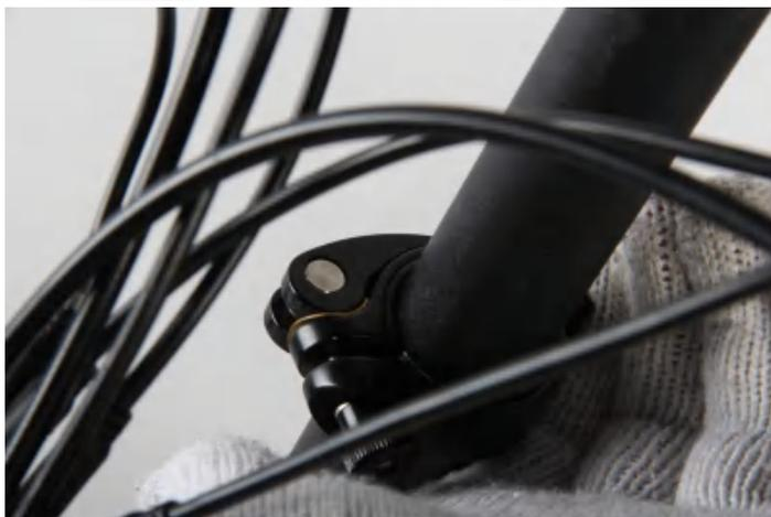
h. Adjust the handlebar horizontal angle as required by lifting up the handlebar stem quick release lever, then twist the handle bar to the correct angle and firmly press the quick release lever down again to lock.
