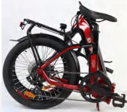
**Unfolding:** Unfold the main frame until the hinge joint is fully closed and lock it by pushing alloy lock lever until it clamps against the frame. Ensure the Safety catch clicks into position and the lever cannot open.
