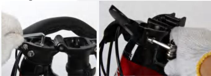
b. Carefully unfold the handlebar stem post up into its vertical position, Rotate the handlebars to sit perpendicular to the front wheel. Once satisfied the bars are correctly aligned, fold the bars down (without twisting) and retighten the stem screws.
